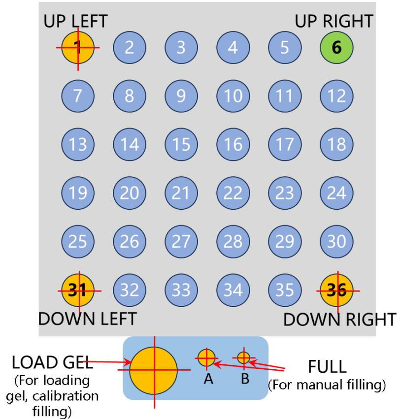
Note: The UP RIGHT position does not need calibration. This position will be automatically completed based on the UP LEFT, DOWN LEFT, and DOWN RIGHT three positions.
