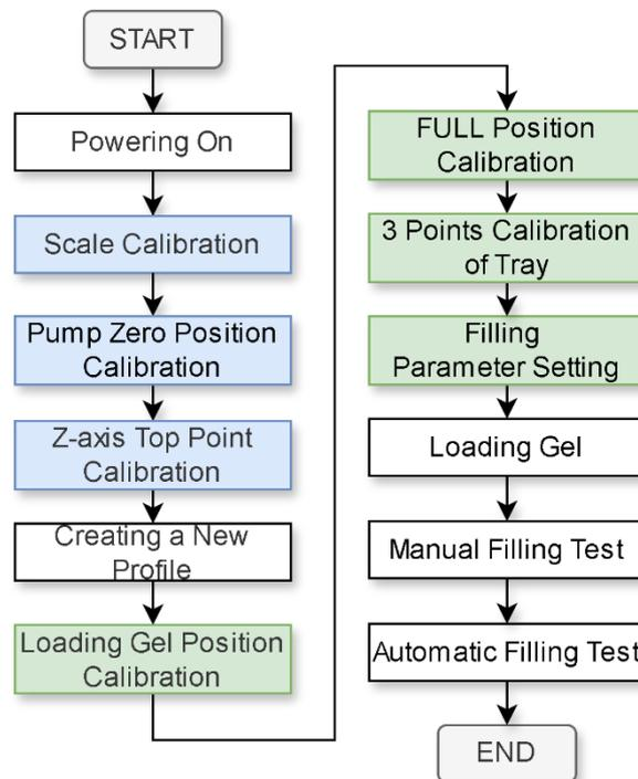
Note: After switching to a new bottle profile, large and small scale calibration, pump zero point calibration, and Z-axis top point calibration can be optionally performed.
